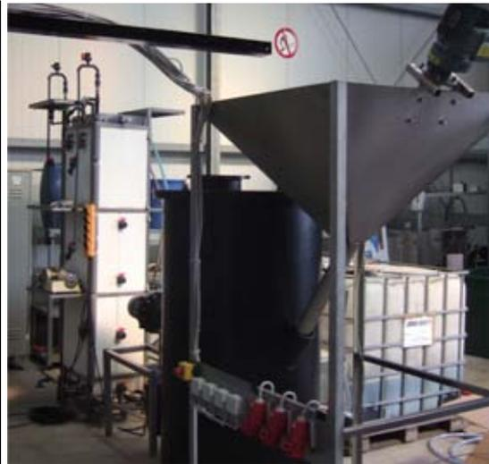
Fig. 7: Test plant TiHo 5 m<sup>3</sup> hydrolysis,
