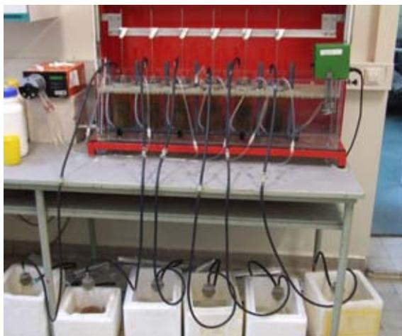
*Fig. 4: Rumen simulation technique (Rusitec) TiHo*
