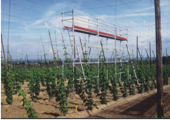
Fig. 1. Scaffold tower for the field monitoring of aphid migration and aphid population development. Oberulrain, Bavaria, Germany, May 1996.
