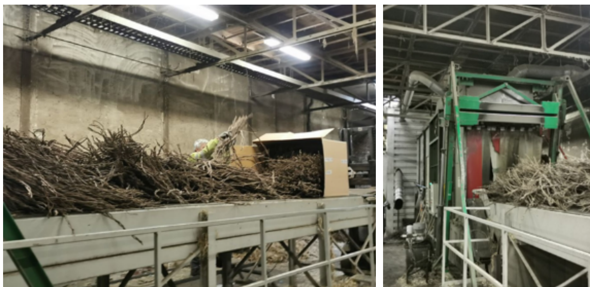
Figure 19 Moisture dosing of the test material into the wood separation process of HempFlax Group B.V. in Oude Pekela (NL)
