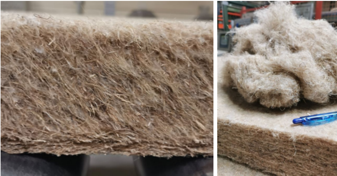
Figure 27: Finished insulation mat made from 30% hops, 60% hemp, and 10% bonding fiber material, compared to the starting fiber material (right)
