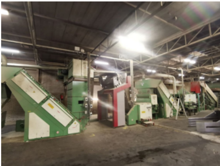
Figure 20: Fiber cleaning and fiber opening line at HempFlax; (left, middle and right step cleaner, fiber opener in between)
