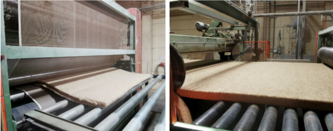
Figure 26: Thermally compressed insulation mat (left) and width calibration (assembly) of the product (right)
