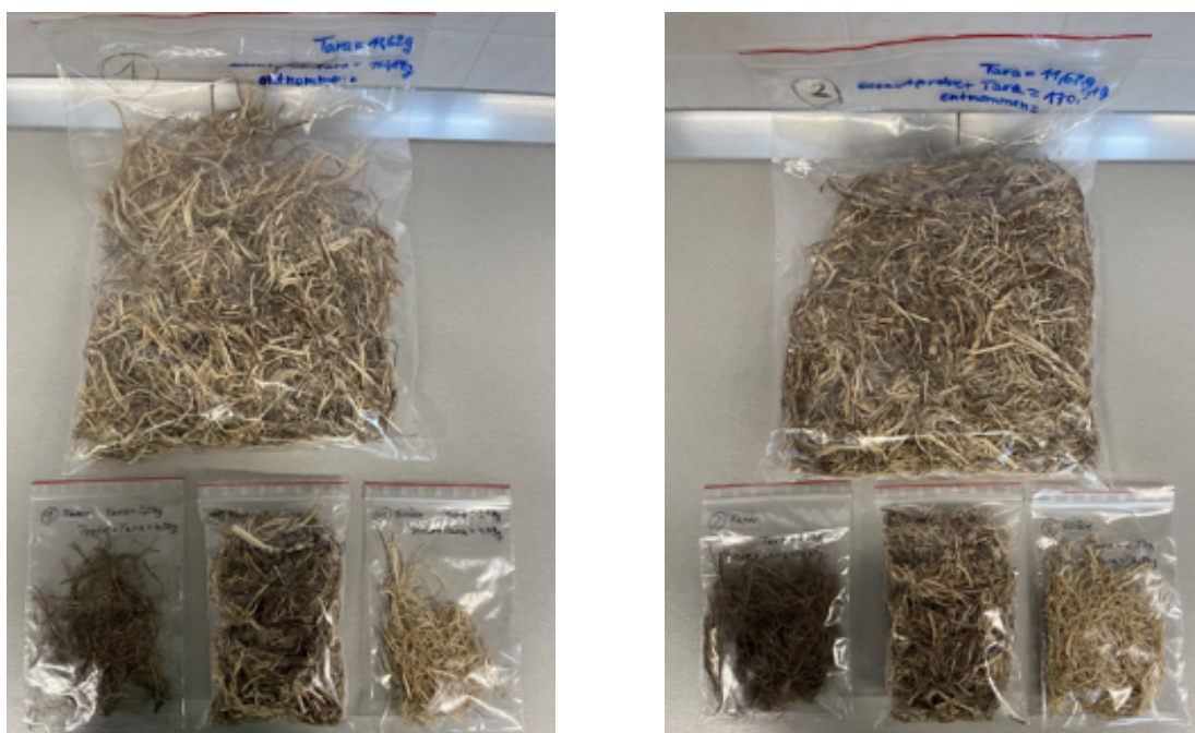
Figure 21: Experimental samples of hop stems (top of each), as well as fractions selected from them (at the bottom left, pure fiber bast; in the middle, fiber bast with firmly adhering shives; and on the right, pure shives)
