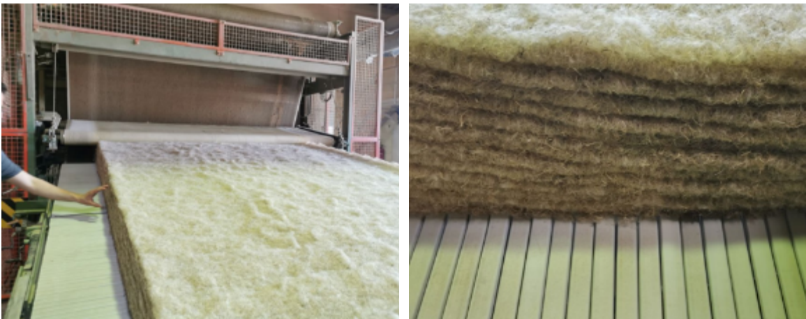
Figure 25: Multi-layer pile before thermal solidification
