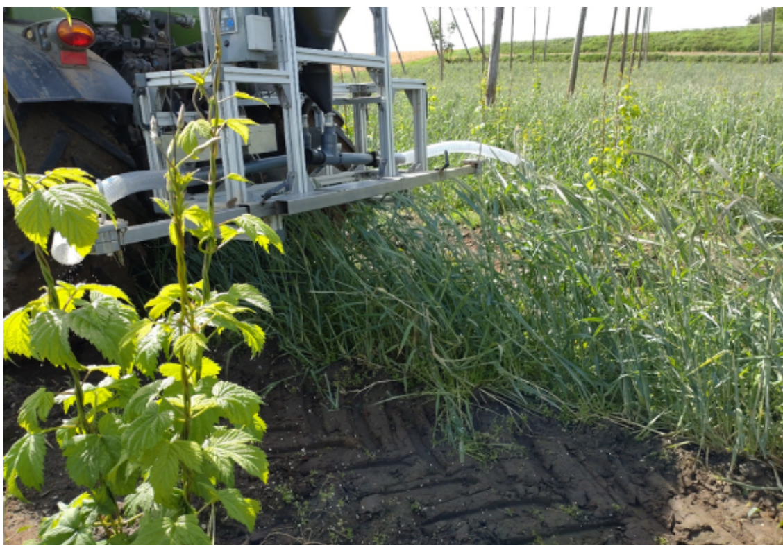
Figure 85: Using sawdust as a carrier substance, the predatory mites are gently blown on the young hop bines
