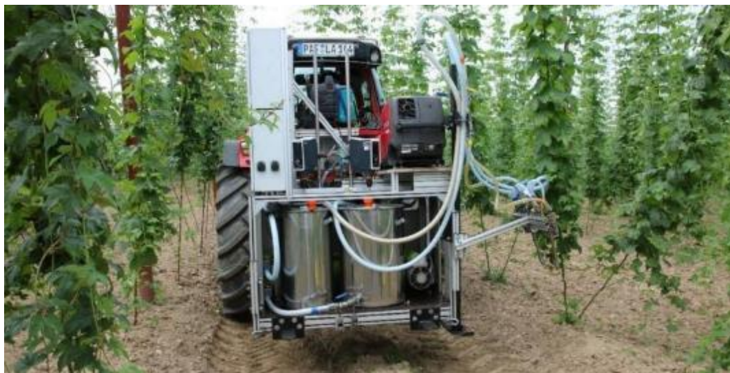
Figure 27: Application device “SAM” (system for the application of mulch material) equipped with one tank per component, a separate piping system, and a mixer for application in the furrow
