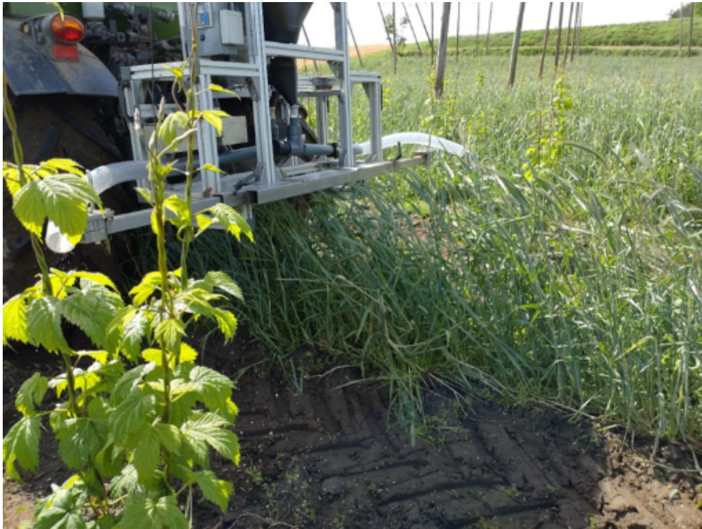
Figure 77: Using sawdust as a carrier substance, the predatory mites are gently blown onto the young hop bines during application
