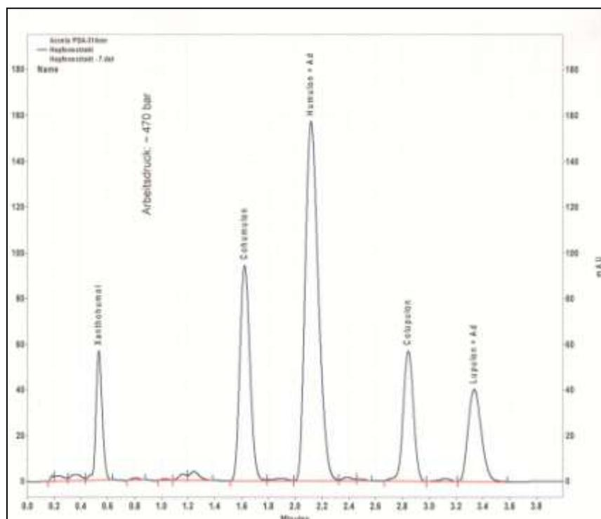
Fig. 7.1: Bitter-compound chromatogram with a 100 mm, 1.9 µm column
