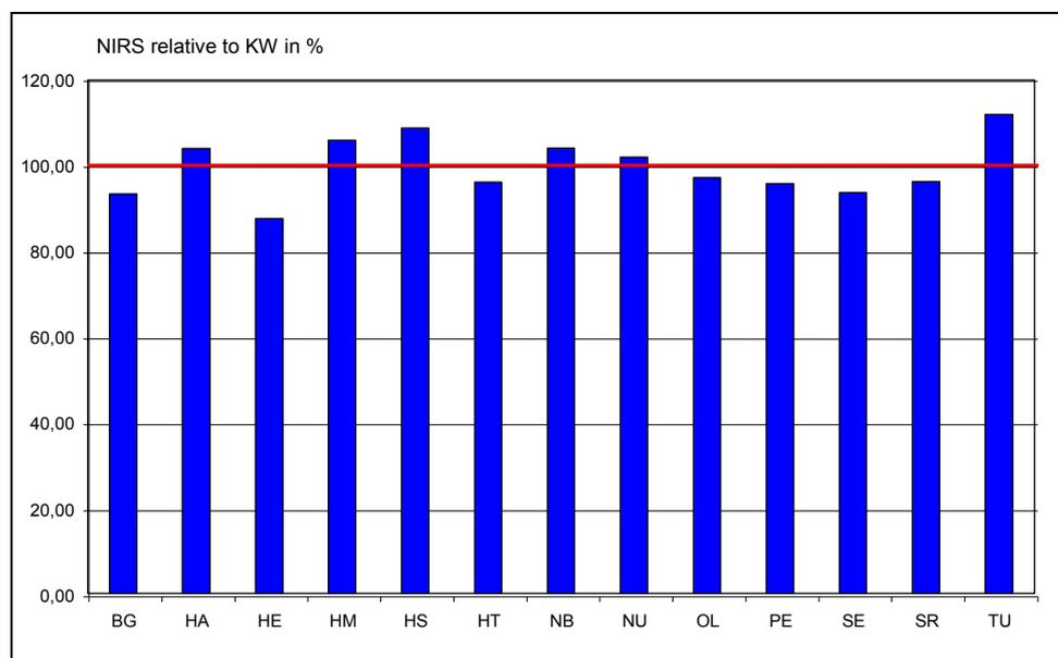
Fig. 7.4: NIRS values relative to conductometric values for the 2008 crop
