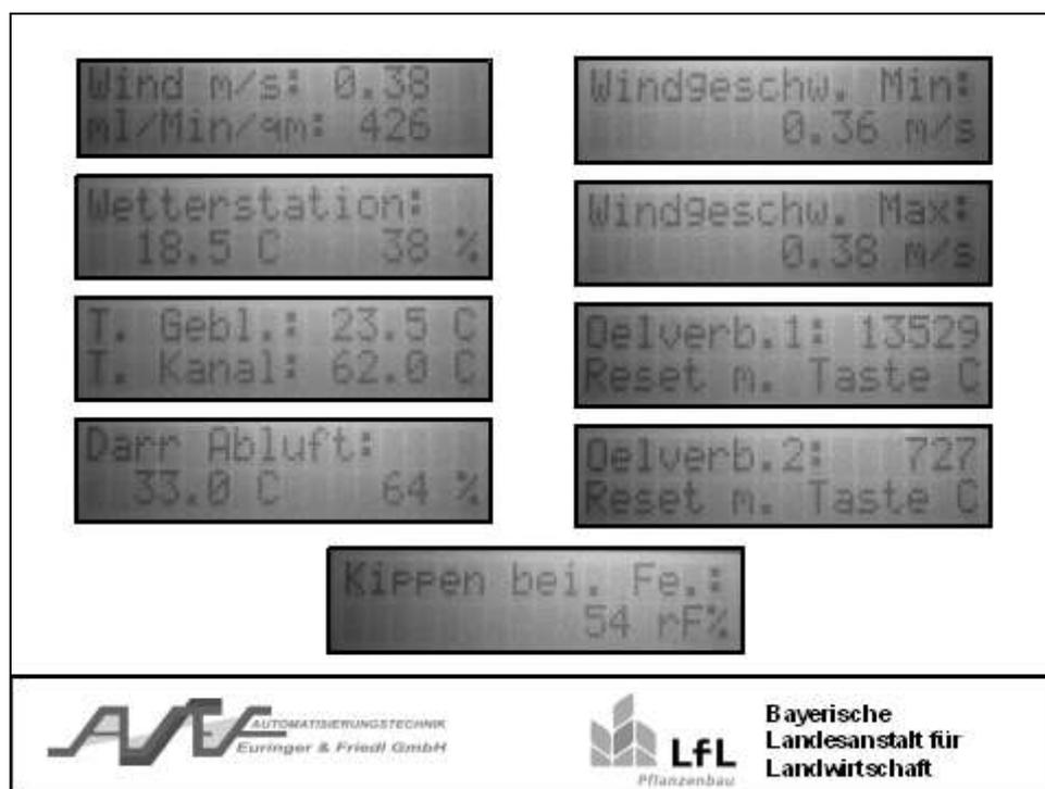
Fig. 5.3: Sample display of practice-oriented drying parameters supplied by the newly developed measuring system.
