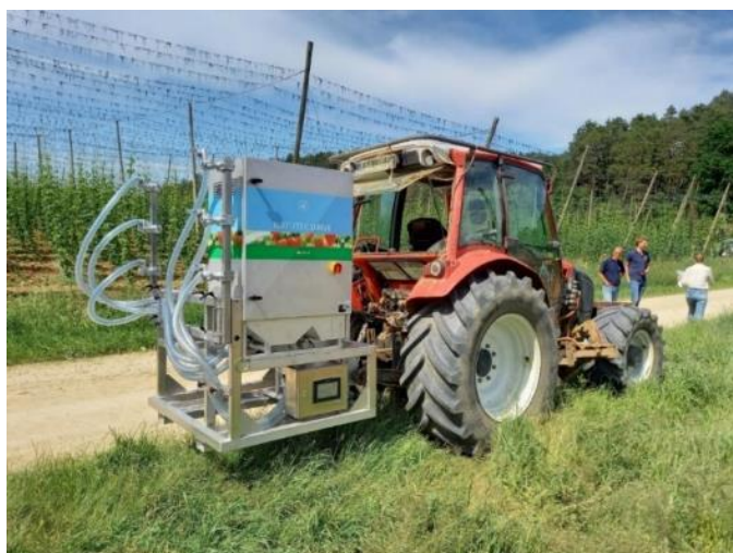
Figure 8.4: Novel construction by Koppert ('Natutec') for the release of predatory mites in hops; Dürnwind, June 2021
