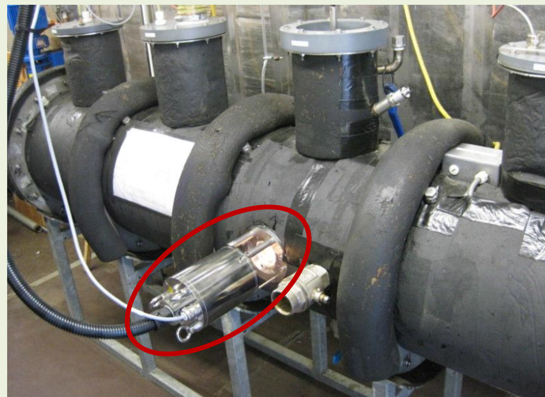
Fig. 1 240 liter laboratory digester, NIR-sensor (Bruker)
