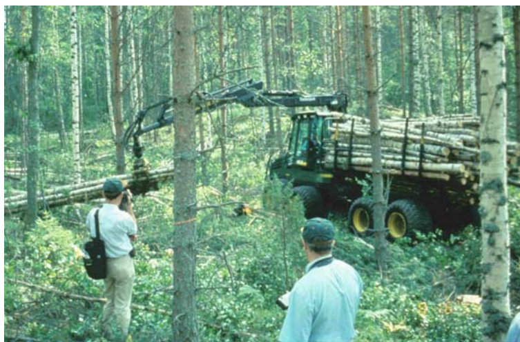
Abb. 13: Forwarder (Trag-Knickschlepper, Kranrückezug)
