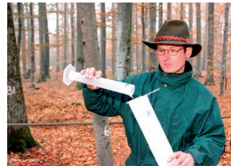
The local forest officer takes a throughfall sample for laboratory analysis of nitrogen deposition.
